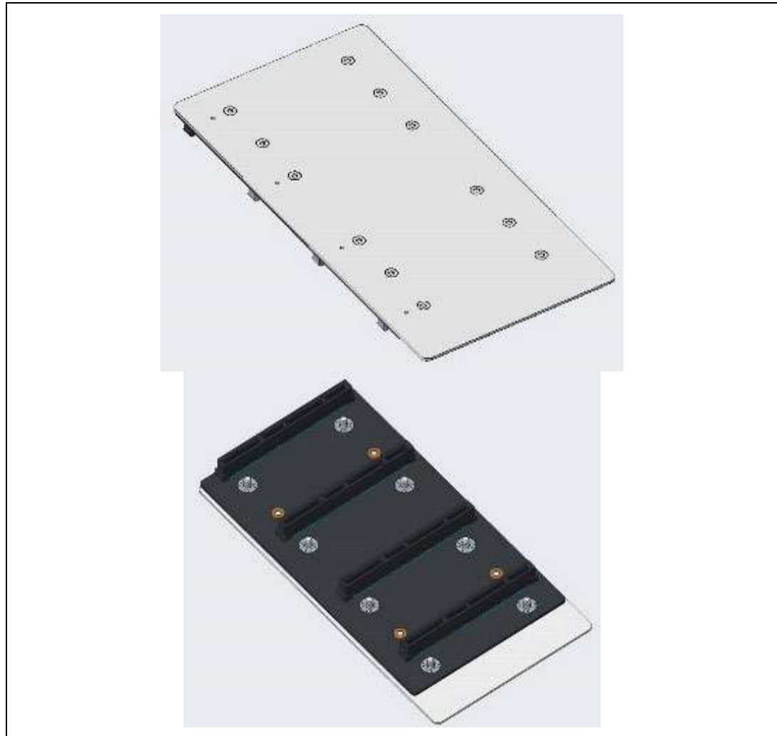
Figure 3-7. Four-Card Intel X e Link Bridge Connector
