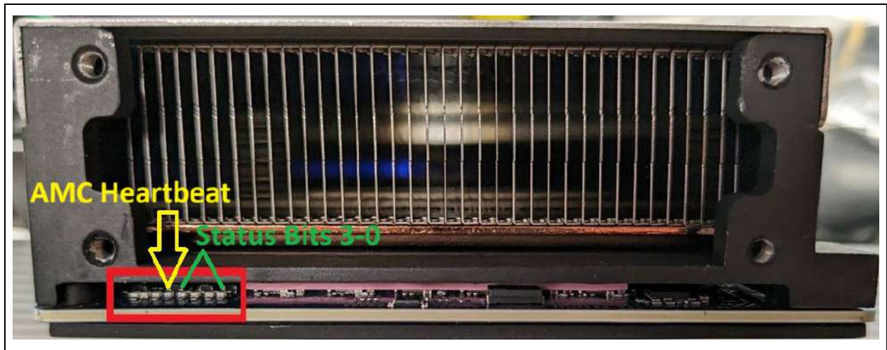
Figure 7-4. Debug and Card Status LED Location (I/O Bracket Removed)
